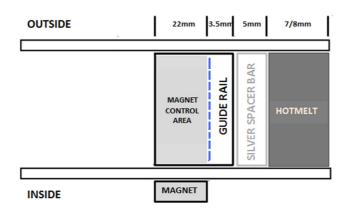
PLEASE NOTE - it is important that when measuring sealed units allowance is made to ensure the magnets sit in their correct positions (where guide rails are fitted) and have the overlap of 20mm.
